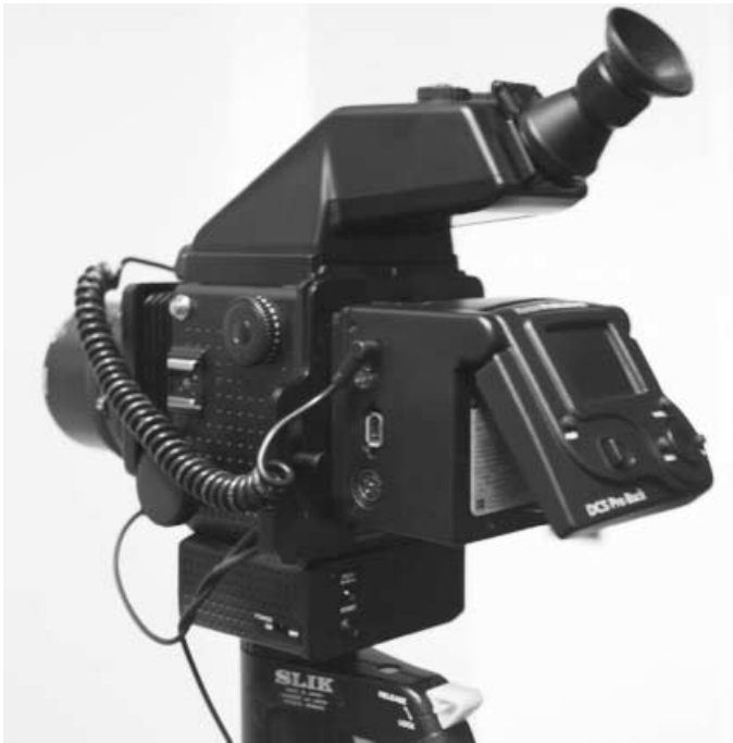
FIG. 1. Kodak DCS Pro Back mounted onto the Mamiya RZ67 Pro II camera body.
