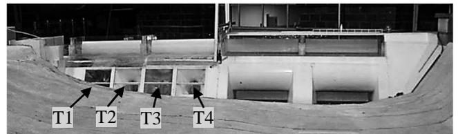
Figure 1: A photograph with the HPP model structure; there are 4 intakes on the left bottom, 2 outlets on the right bottom and 4 flap gates on the top part of the plant.
